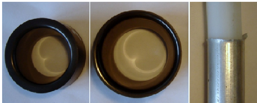
Outer conductor of coaxial cable
